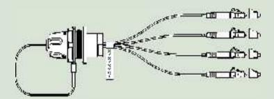
In our standard offer, each cable assembly is identified with a wire marking sleeve (Brady material B-342).
